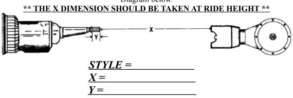
X measurement will be from the tip of the output shaft to the center line of the universal joint or flat of the flange on most all 2wd vehicles. Y measurement will be how far the output shaft protrudes from the seal.
